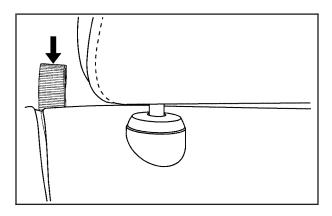
To lower the rear seatback, pull on the seat tab located on the outboard side of the seatback cushion and fold the seatback down. This allows you direct access to the trunk.
